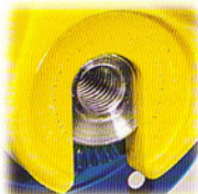
D-shaped axle end prevents rotation of the fork blades around the axle center*
