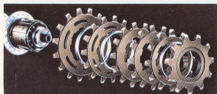
Spline-type cassette gear of Dura-Ace EX Freehub.
