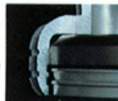
Sectional View of Rotating Head Part (Labyrinth Seal)
