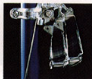
Trapezium shaped swing motion of Trap-Ease Mechanism.
